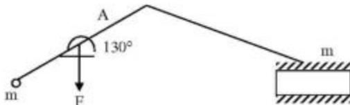
37. An offset slider-crank mechanism is shown in the figure. Conventionally, the Quick Return Ratio (QRR) is considered to be greater than one. The value of QRR is \_\_\_\_\_
