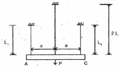
17. A rigid bar AC is supported by three rods of same material and of equal diameter. The bar AC is initially horizontal. A force P is applied such that the bar AC continues to remain horizontal. Forces in each of the shorter bars and in the longer bar are, respectively.
