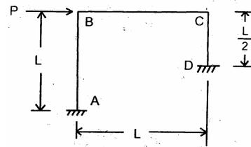
48. A portal frame with all member s having the same  $EI$ , has one end fixed and the other hinged. Due to side-sway, the ratio of fixed end moments  $M_{BA} / M_{CD}$  would be
