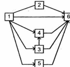
99. A-O-A network is suggested as shown above. The number of errors/incompatibilities in this network is
