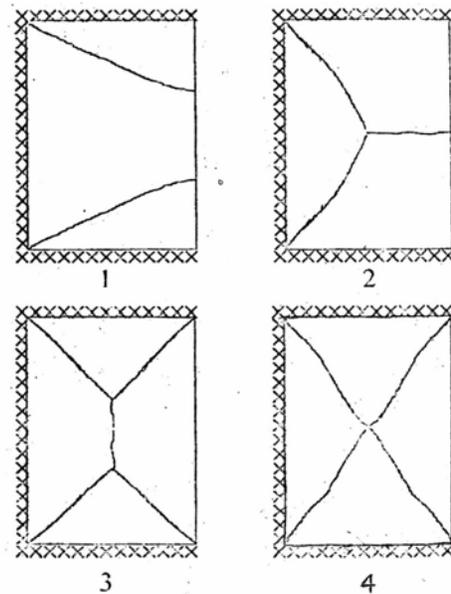
A reinforced concrete rectangular slab is built-in (fixed) on three edges and the other edge is free. The possible yield line patterns for the slab subjected to a uniformly distributed load and reinforced isotropically are shown above as 1, 2, 3 and 4.
