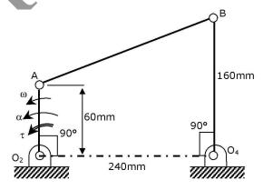
76. Which kind of 4-bar mechanism is 02AB04?
