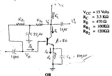
Sketch an RC coupled Amplifier circuit which is operated a) in the CE configuration & explain how this circuit operates as an amplifier. Draw the input base signal, collector current & collector voltage waveform. Indicate how you can draw the load line (DC') for the circuit you have drawn.
