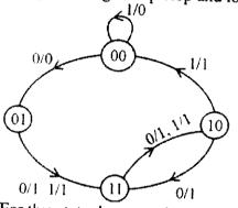
For this state diagram, design a circuit using J-K flip-flops and logic gates
