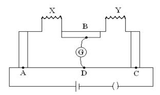
The figure shows experimental set up of a bridge. When the two unknown resistances X and Y are inserted, the null point D is obtained 40 cm from the end A. when a resistance of 10 is connected in series with X, the null point shifts by 10 cm. find the position of the null point when the 10 resistance is instead connected in series with resistance 'Y'. Determine the values of the resistances X and Y.
