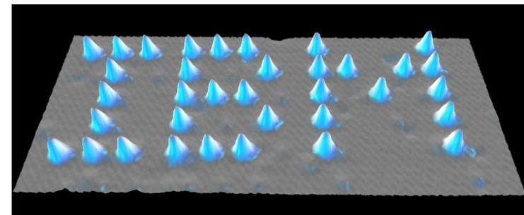
**Positioning single atoms with scanning tunneling microscope (Xe on Ni). Eigler, IBM, 1990.**
