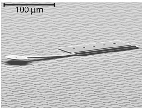
**World’s smallest mobile robot, with no wheels, gears or hinged joints**
