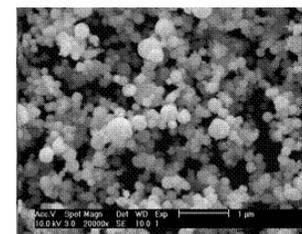
Nanoparticles by flame pyrolysis (Princeton)
