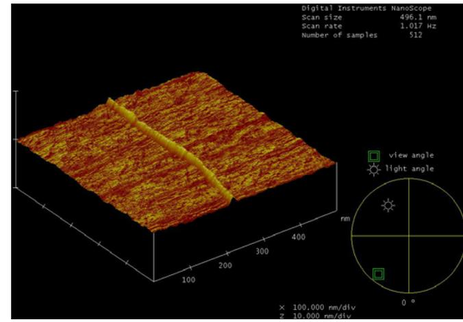
**AFM image of carbon nanotube**
