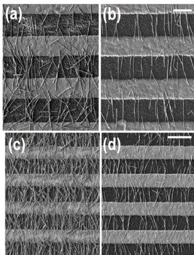
Electric field aligning of nanowires (U. Mass)
