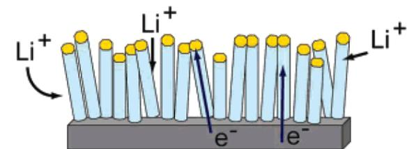
**Si or Ge nanowire batteries holding 10 times the charge of existing lithium-ion batteries** (Stanford)
