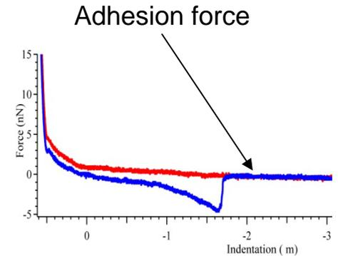
AFM force measurements of the tip interaction with the bilayer.
