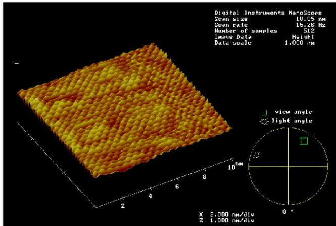
**AFM image of mineral surface showing atomic structure.**
