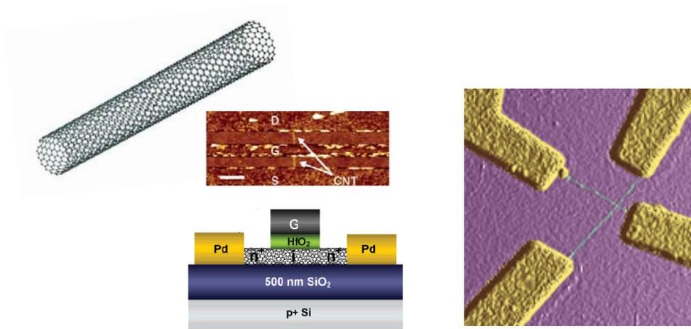
**Carbon nanotube (CNT) transistor for future computer chips** (Stanford, UC Berkeley)
