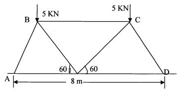
Analyze the frame by method of joints and method of sections.
