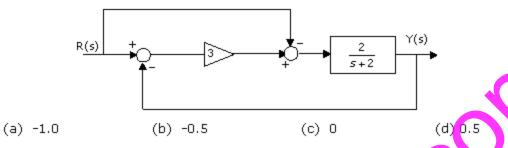
In the GH(s) plane, the Nyquist plot of the loop transfer function 39.
