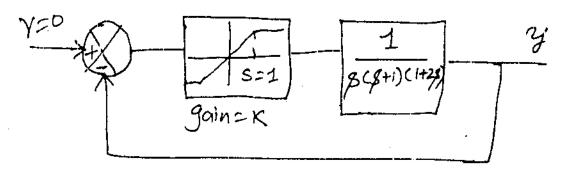
(b) Using Second Method of Liapunov, examine the stability of the System 10 given by—
