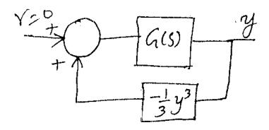
Also calculate describing function of  $f(y) = \frac{1}{3}y^3$ . And Estimate, The frequency and amplitude of possible limit cycle.
