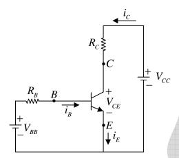
and the leakage current is negligible. What is the required value of  $R_B$  in kilo-ohms if the base current is to be  $4 \mu A$ ?
