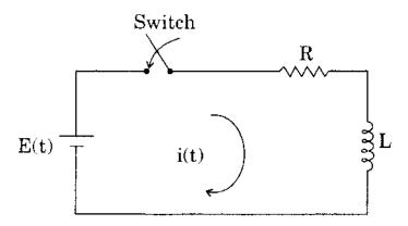
(b) In the circuit shown in figure,  $R=5~k\Omega$ , the relay is adjusted to operate with a current of  $~7\,mA$ . The switch is closed at t=0 with initial current i(0) = 0. It is found that the relay operate at t=0.2~sec. Find the inductance L of the relay coil.
