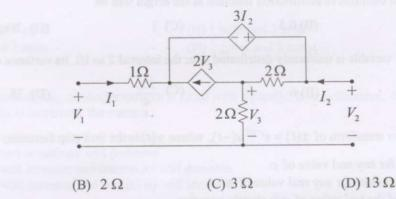
Q.31 In the circuit shown below the average power consumed by the  $1\Omega$  resistor is
