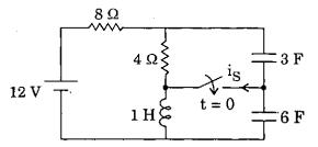
In the circuit shown above, the switch is closed after a long time. The current  $i_S$  (0<sup>+</sup>) through the switch is
