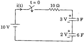
In the circuit shown above, switch S is closed at t = 0. The time constant of the circuit and initial value of current i(t) are
