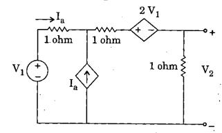
The above network contains resistors and controlled sources.  $G_{12} = \frac{V_2}{V_*}$  is
