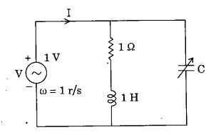
In the above circuit, the value of C for the circuit to exhibit a power factor of 0.86 is approximately
