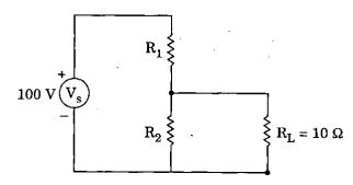
What is the voltage across the load resistance,  $\boldsymbol{R}_L$  in the above circuit ? The value of each resistor connected in the circuit is 10  $\Omega.$
