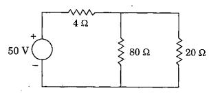
The value of current in 80  $\Omega$  resistor of above circuit is
