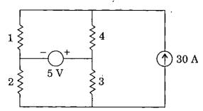
The power dissipated in the 1  $\Omega$  resistor is 1 W due to the 5 V voltage source alone and 576 W due to 30 A current source alone. The total power absorbed in the same resistor due to both the sources is
