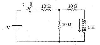
The value of V that would result in a steady-state current of 1 A through the inductor in the above circuit is
