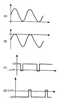
20. A single-phase half wave uncontrolled converter circuit is shown in figure. A 2-winding transformer is used at the input for isolation. Assuming the load current to be constant and  $v = V_m \sin \omega t$ , the current waveform through diode  $D_2$  will be
