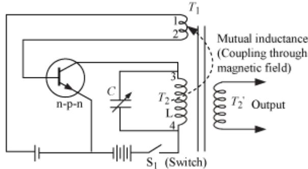
In an oscillator, a sustained A.C. output is obtained without any input oscillation. For this to happen, the output of a transistor amplifier is fed back into its input. This is achieved by coupling the winding  $T_1$  to winding  $T_2$ .
