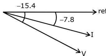
I lead V so it is a combination of Resistance and capacitance
