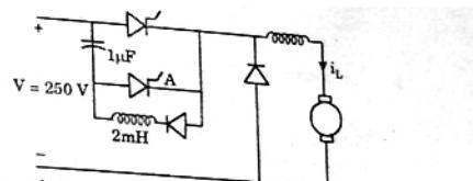
84. The minimum time in  $\mu$ sec for which the SCR M should be ON is
