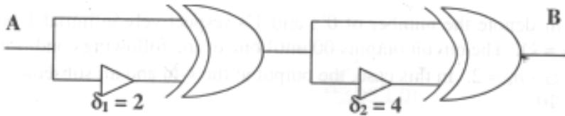
The non-inverting buffers have delays  $\delta_1 = 2$  ns and  $\delta_2 = 4$  ns as shown in the figure. Both XOR gates and all wires have zero delay. Assume that all gate inputs, outputs and wires are stable at logic level 0 at time 0. If the following waveform is applied at input A, how many transition(s) (change of logic levels) occur(s) at B during the interval from 0 to 10 ns?
