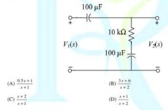
Q.3 Assuming zero initial condition, the response y(t) of the system given below to a unit step input u(t) is
