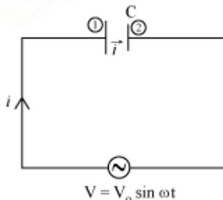
When a capacitor is connected to an alternating current, it offers a resistance  $X_c \left( = \frac{1}{\omega c} \right)$  and allows the current to pass through.
