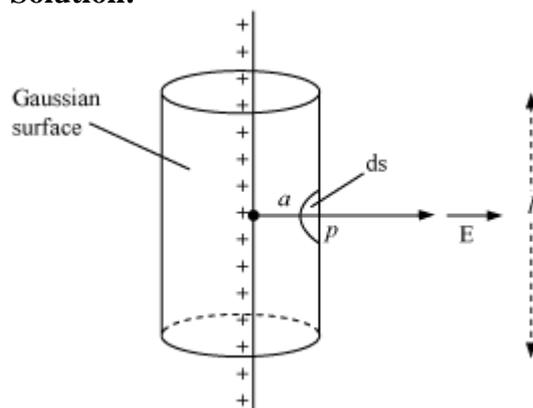
The thin infinitely long straight line has a linear charge density  $\lambda$ .
