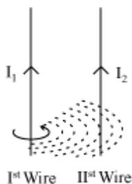
Magnetic field  $\vec{B}$ , will be moving into the page and  $I_2$  is moving upward on the plane of the page.
