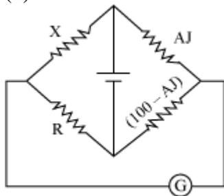
At the balance position there is no current flowing through the galvanometer. Hence, interchanging the battery and the galvanometer will have no effect on the balance point.
