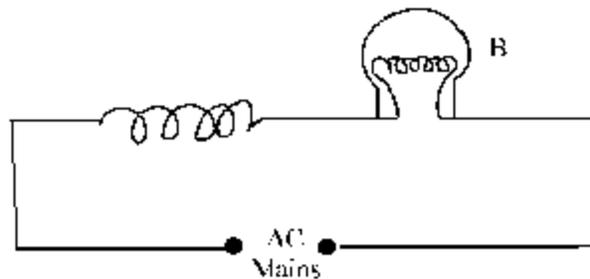
The bulb glows with some brightness. How would the glow of the bulb change if an iron rod were inserted in the coil? Give reasons in support of your answer. 2
