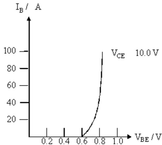
Cut off Stage : When the input voltage is less than a minimum value ( $\approx 0.6$ V for Si), there is no current flow in the input or output sides of the transistor. The transistor is then said to be in its 'cut-off' stage. 1
