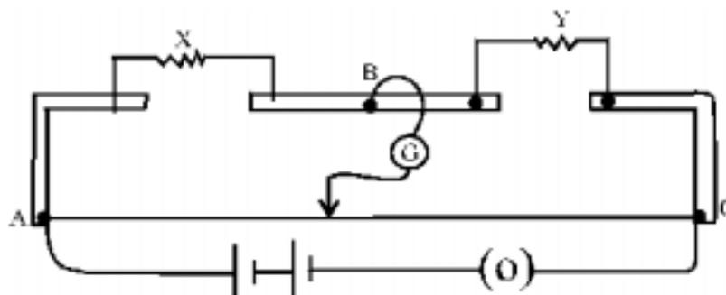
When a resistance of  $15 \Omega$  is connected in series with 'Y', the null point is found to shift by 10cm towards the end A of the wire. Find the position of null point if a resistance of  $30 \Omega$  were connected in parallel with 'Y'. 3
