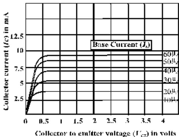
Use these graphs to obtain the approximate value of current amplification factor for the transistor at  $V_{CE} = 3V$ . 3
