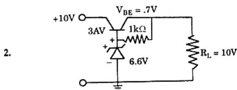
$$\text{Current in } R_L = \frac{6.6 - 0.7}{10} = 0.59 \text{ amp}$$
