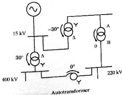
Equal phase shift of points A and B with respect to source from both bus paths.
