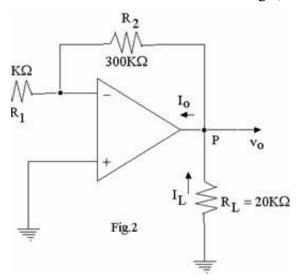
c. Draw the circuit of an OPAMP V-to-I converter with grounded load and derive the equation for the current through the load. (6)
