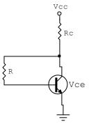
Derive the transfer caracterstics in terms of R, I<sub>s</sub> (I<sub>s</sub> being the reverse saturation current of the transistor) and  $V_T$ . Assume n=1.
