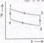
An ideal gas completes a cycle consisting of two isotherms and two isochors as shown in the above figure. Which one of the following is correct?
