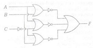
Which one of the following gives the output F for the logic diagram shown above?
