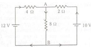
What is the value of current passing through the brance AB in the electric circuit given above?
