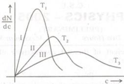
The plots of Maxwell's distribution function  $\left(\frac{dN}{dc}\right)$
