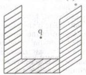
A charge q is placed symmetrically with respect to three faces of equal area as shown in the figure given above. What is the total electric flux through the faces?
